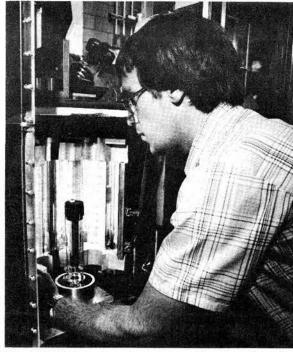
FURNACE for the laser interferometric dilatometer opens for sample placement. Containing four quartz lamps, the cloverleaf-shaped aluminum chamber has polished reflective surface, can heat samples to 900 K.
